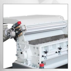
Efficient grinding thanks to the fixed knives at 0°
