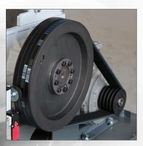
Keys for the fixing of motor pulley and fly-wheelPulley and fly-wheel design gives higher inertia
